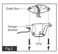
Tighten the hanger bracket to the outlet box with 2 mounting screws. (To reduce the risk of fire, electric shock, or personal injury, mount to the outlet box marked "Acceptable for fan support" and use mounting screws provided with the outlet box.)
