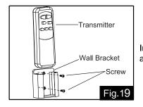
Install the transmitter wall bracket in wall by two screws and hang transmitter in it carefully.
