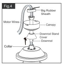
Thread the motor wires through the Downrod Stand Cover, Canopy, Downrod and Big Rubber Sheath.
