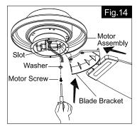
Rotate the motor to remove the motor screws and washers through a slot from the fan motor assembly. Secure blade brackets to the motor with washers and motor screws through a slot.
