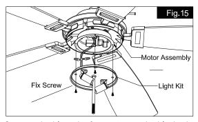
Connect the blue wire from motor to the black wire from light kit by wire connectors. And connect the white wire from motor to the white wire from light kit by wire connectors. Remove one fix screw from bottom of motor assembly (for later use), and loosen the other three fix screws. Secure the light kit to motor assembly with previous fix screw and tighten the other three fix screws.
