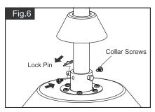
Tighten the two Collar Screws. Slide Lock Pin into Hanger Pin until it is locked into position.
