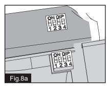
Code example: 1-ON 2-OFF 3-ON 4-OFF on both DIP Switches. Note: If you have two ceiling fans with 2 remote control units, set 2 different codes for each set of transmitter / Receiver.
